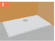
Locate ShowerDec® in the corner to which it is going to be finally positioned & mark lines around the outer edge.
