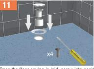
Once the floor coving is laid, screw into position the traps clamping ring using the bolts provided ensuring the inner cup and dip tube can still be
