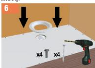
Attach flange to the trap body using the 4 bolts provided, ensuring that the rubber seal is in place. Secure flange to ShowerDec®, there are 4 countersunk indentations in the flange to
